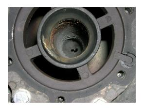
Corrosion in the shot tube of the valves – obviously affected by corrosive flue gas.
