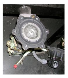
All 9 valves and valve diaphragm are in good condition and require no replacement. Clear result of AEROVIT's patented system with cooling air.
